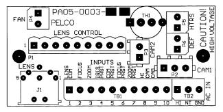
Figure 3. PC Board Component Locations
